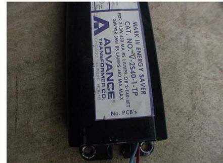
2. **PCB-Containing Ballasts: Intact Ballasts.** An intact light ballast is one that is not (or has not been) leaking any fluids. Many light ballasts will reach the end of their service life without breaching, these are considered to be intact.
