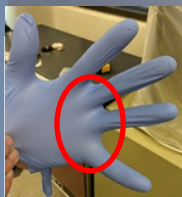
Palm of a stretched nitrile glove showing pinhole breaks in the material.
