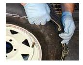
7. Go to the front, take the bow lever, and insert it through the chain link.
