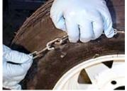
6. On the inner side of the tire, take the "C" hook and hook it through the chain link on the other end of the chains.
