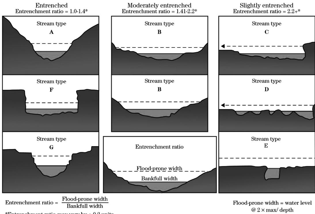
Figure 6. Examples of general channel shape, entrenchment diagrams, and entrenchment ratios for all Rosgen channel types (Rosgen 1996).
