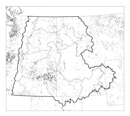
Figure II.12. Each dot represents a recorded dam in the Interior Columbia River Basin (east of the Cascade crest delineated by the heavy line). From Lee et al. 1997. Based on state inventories of dams generally meeting federal regulatory requirements (e.g. > 2m height).
