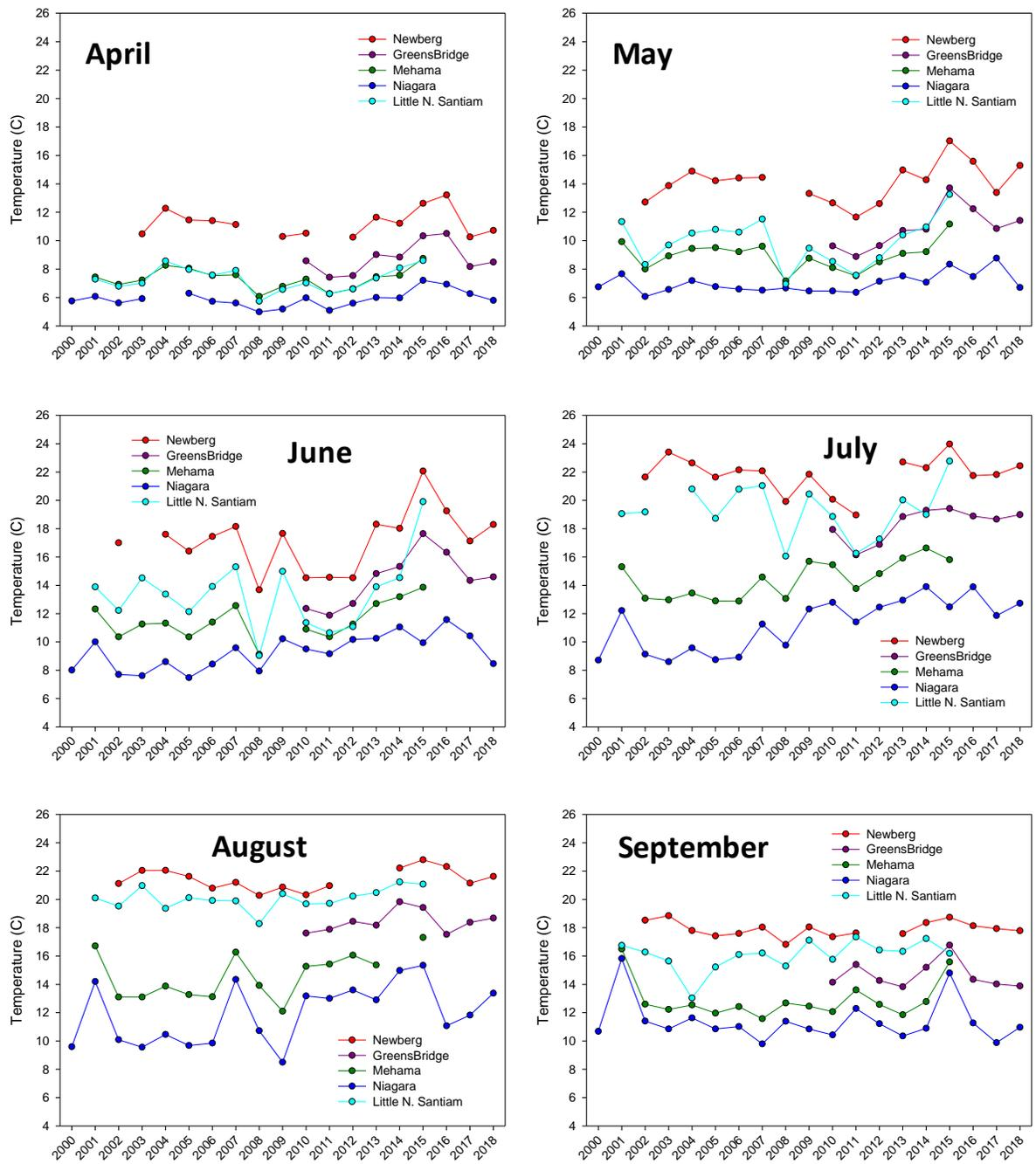
Figure 7. Mean monthly water temperature (°C) at USGS gage sites in the study area, 2000–2018.
