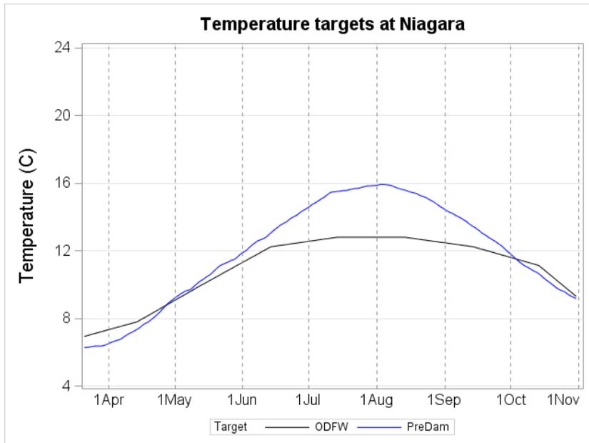
Figure 3. Mean daily water temperature (°C) targets downstream from Big Cliff Dam (at Niagara) that were applied in the temperature management scenarios. Targets were the estimated without-dams (PreDam) temperatures described by Buccola et al. (2012, 2015), and the temperature recommendations for Chinook salmon developed by ODFW in 2017 (ODFW).
