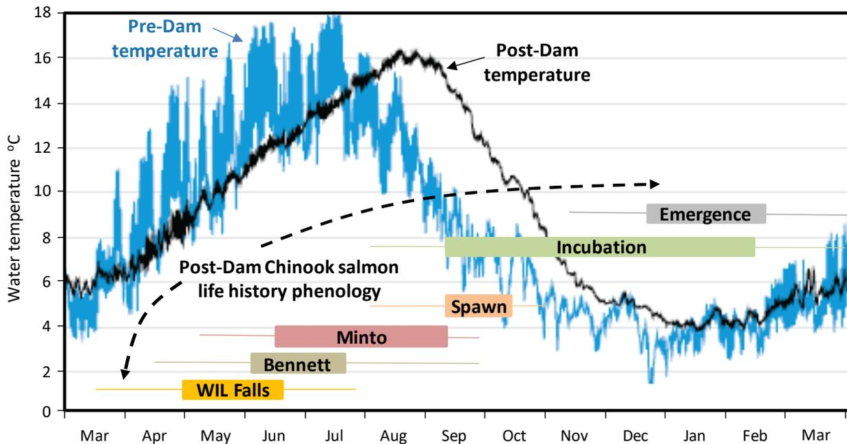
Figure 1. Conceptual diagram showing the effects of Detroit and Big Cliff dams on North Santiam River water temperature (at Niagara), in relation to spring Chinook salmon life history phenology, including adult migration timing at Willamette Falls, the Bennett dams, and at the Minto Fish Collection Facility, spawn timing, egg incubation, and fry emergence timing. Temperature data excerpted from Rounds (2010).
