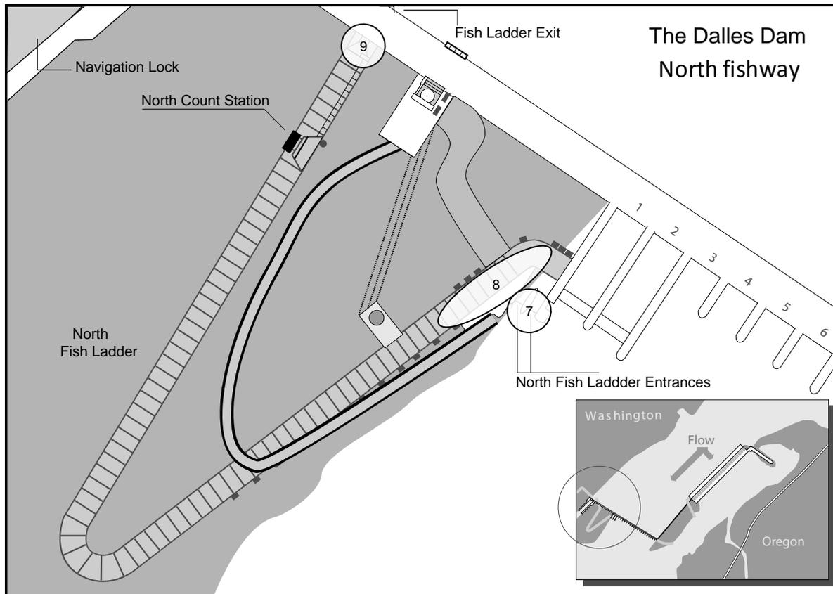
Figure 14. Map of the north fishway at The Dalles Dam. Numbers indicate fishway segments monitored with radiotelemetry.
