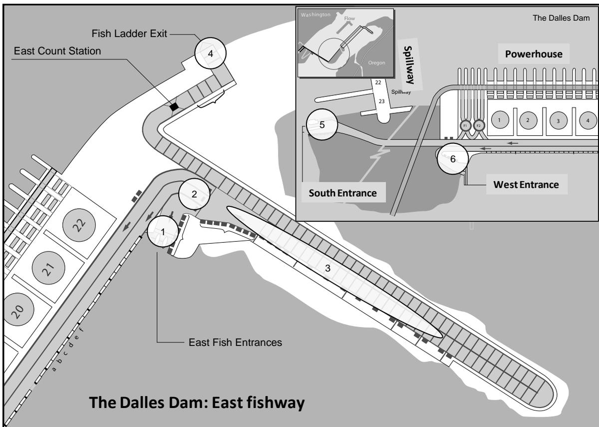
Figure 13. Map of the east fishway at The Dalles Dam. Numbers indicate fishway segments monitored with radiotelemetry.
