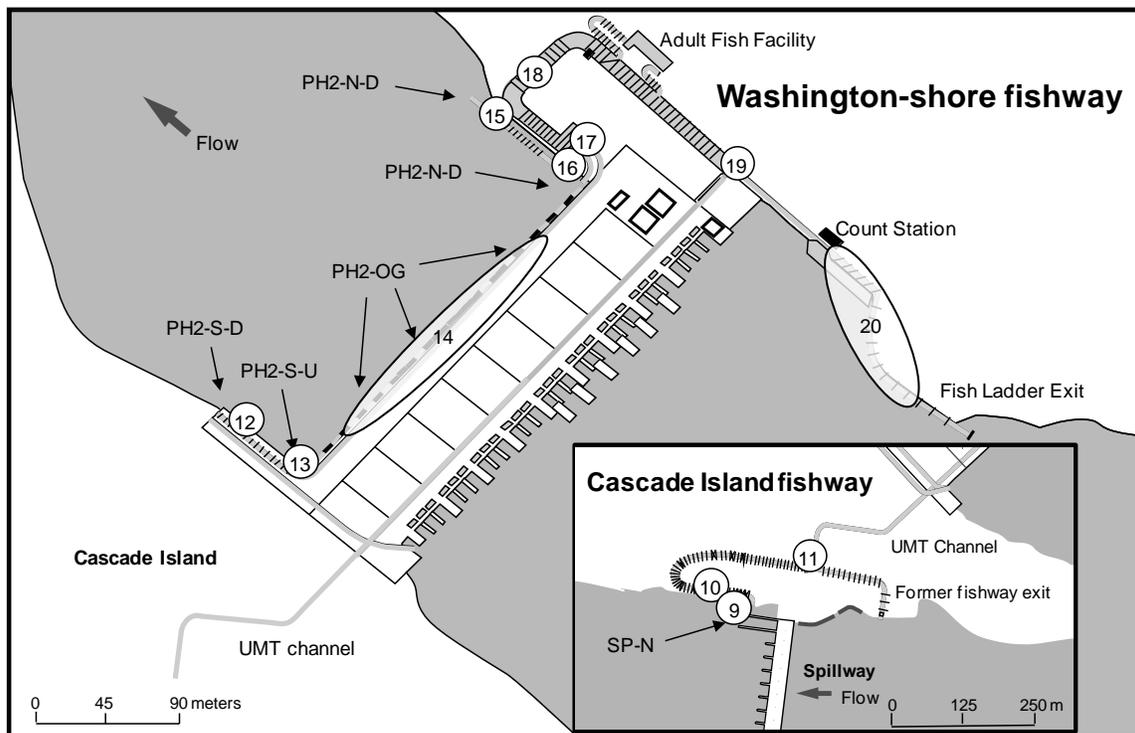
Figure 2. Map of Washington-shore fishway at Bonneville Dam. Numbers indicate fishway segments monitored with radiotelemetry.
