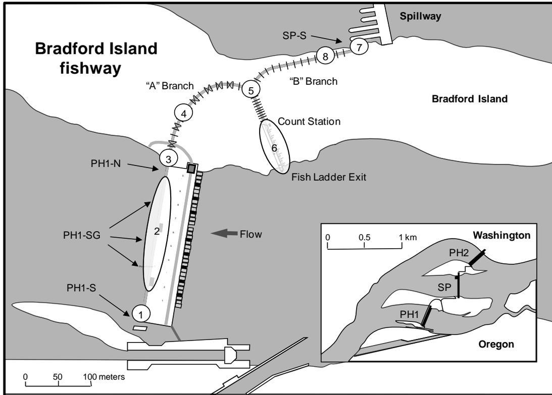
Figure 1. Map of Bradford Island fishway at Bonneville Dam. Numbers indicate fishway segments monitored with radiotelemetry.
