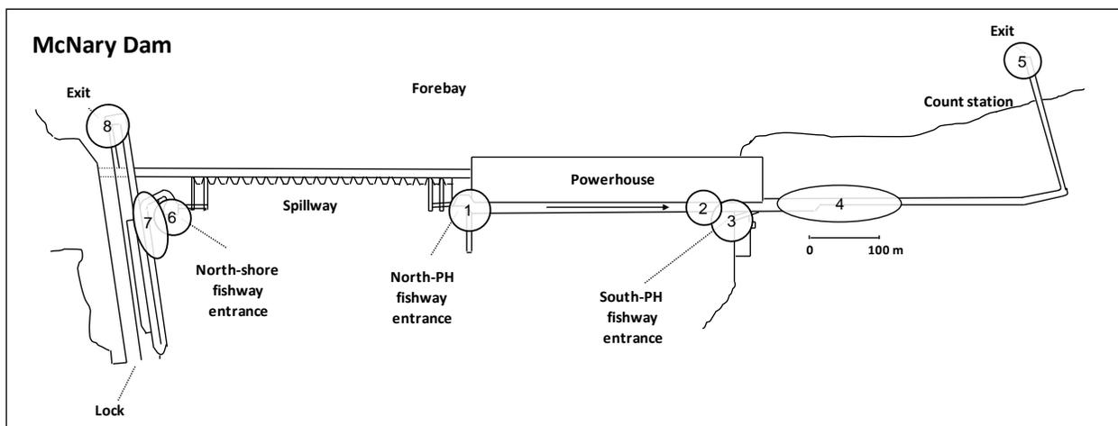
Figure 30. Map of the fishways at McNary Dam. Numbers indicate fishway segments monitored with radiotelemetry.
