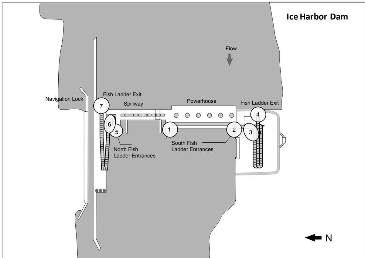
Figure 38. Map of the fishways at Ice Harbor Dam. Numbers indicate fishway segments monitored with radiotelemetry.
