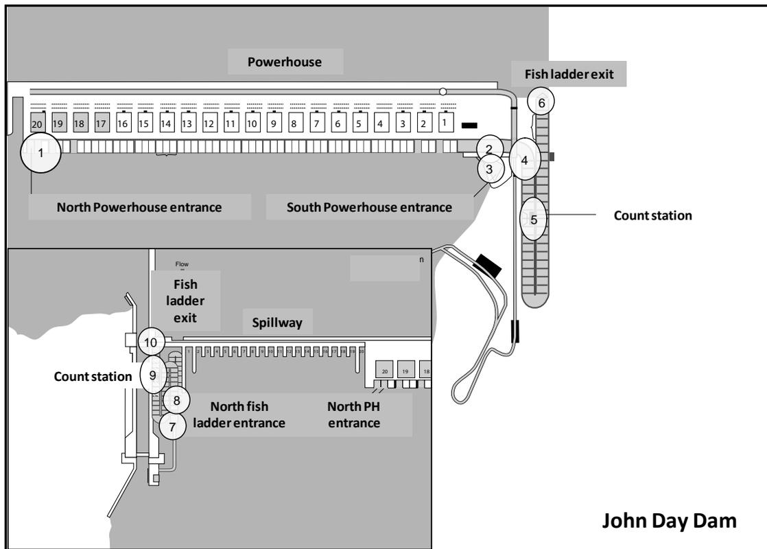
Figure 22. Map of the fishways at John Day Dam. Numbers indicate fishway segments monitored with radiotelemetry.
