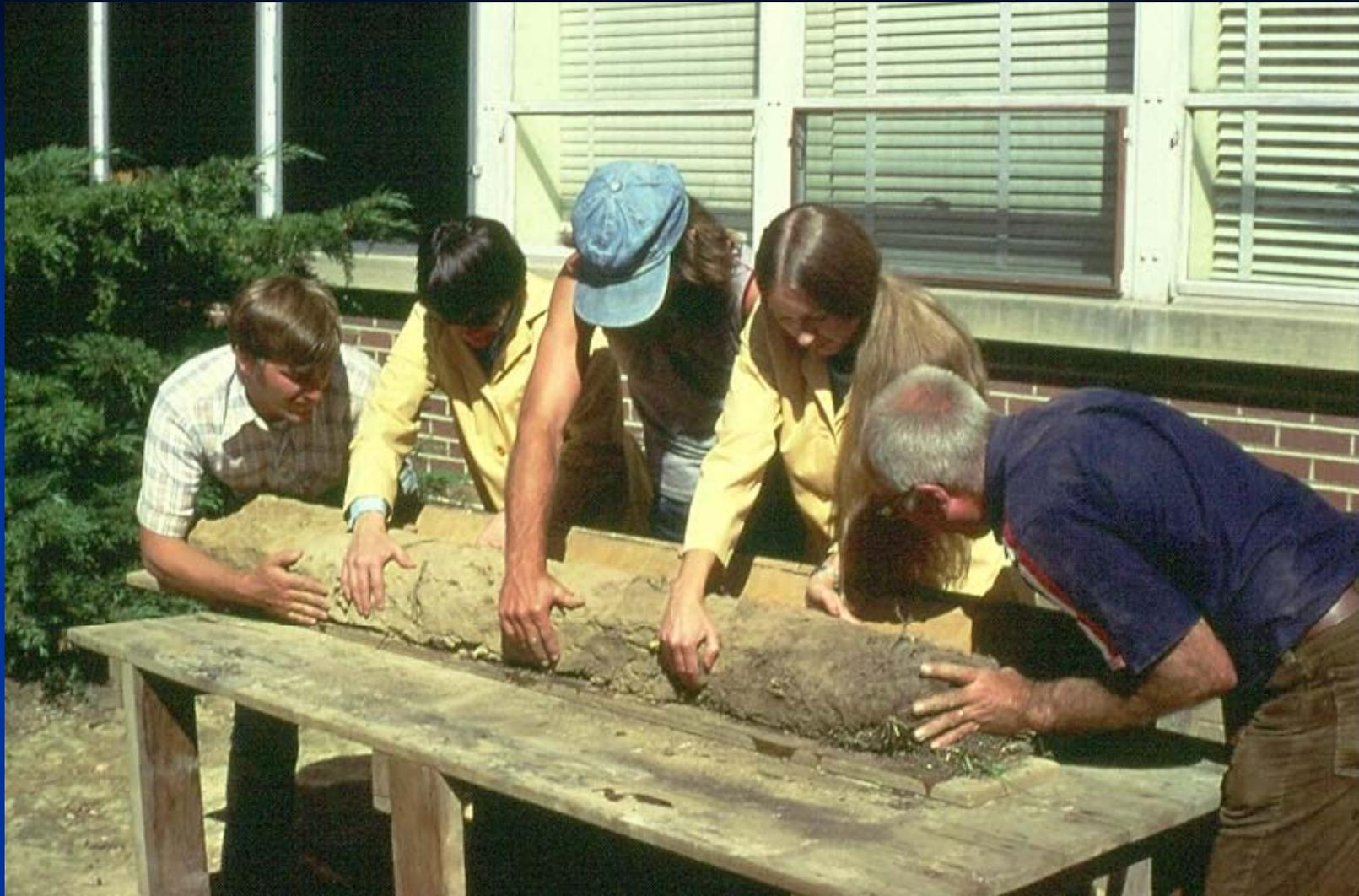
Push the soil into place on the board and close any cracks.
