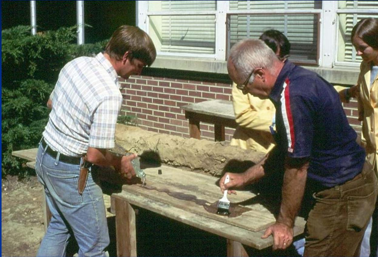
Coat the second board, to which the soil profile is to be transferred, with cellulose.
