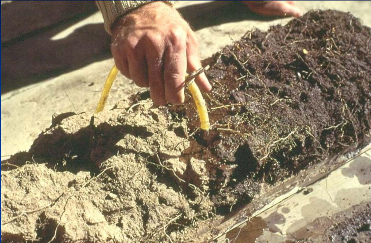
After the soil has dried, soak it with vinylite resin.
