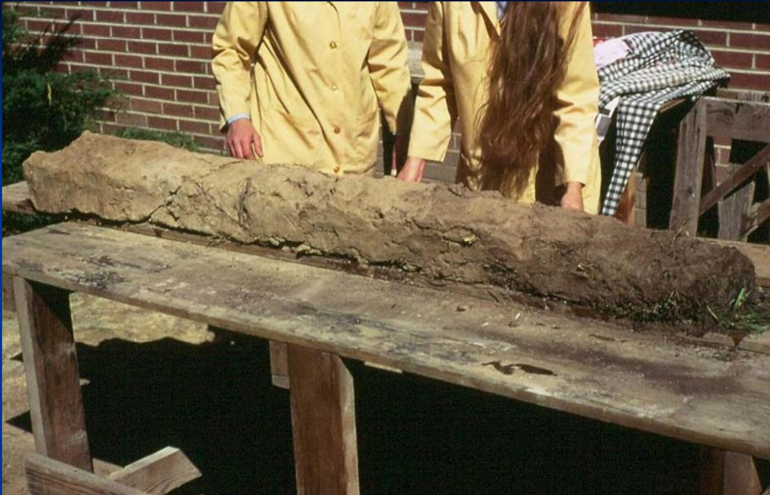
The soil is ready to be worked down with pocket knives and air pressure to expose the structure and achieve the proper thickness. The soil must be moist or this step cannot be accomplished.
