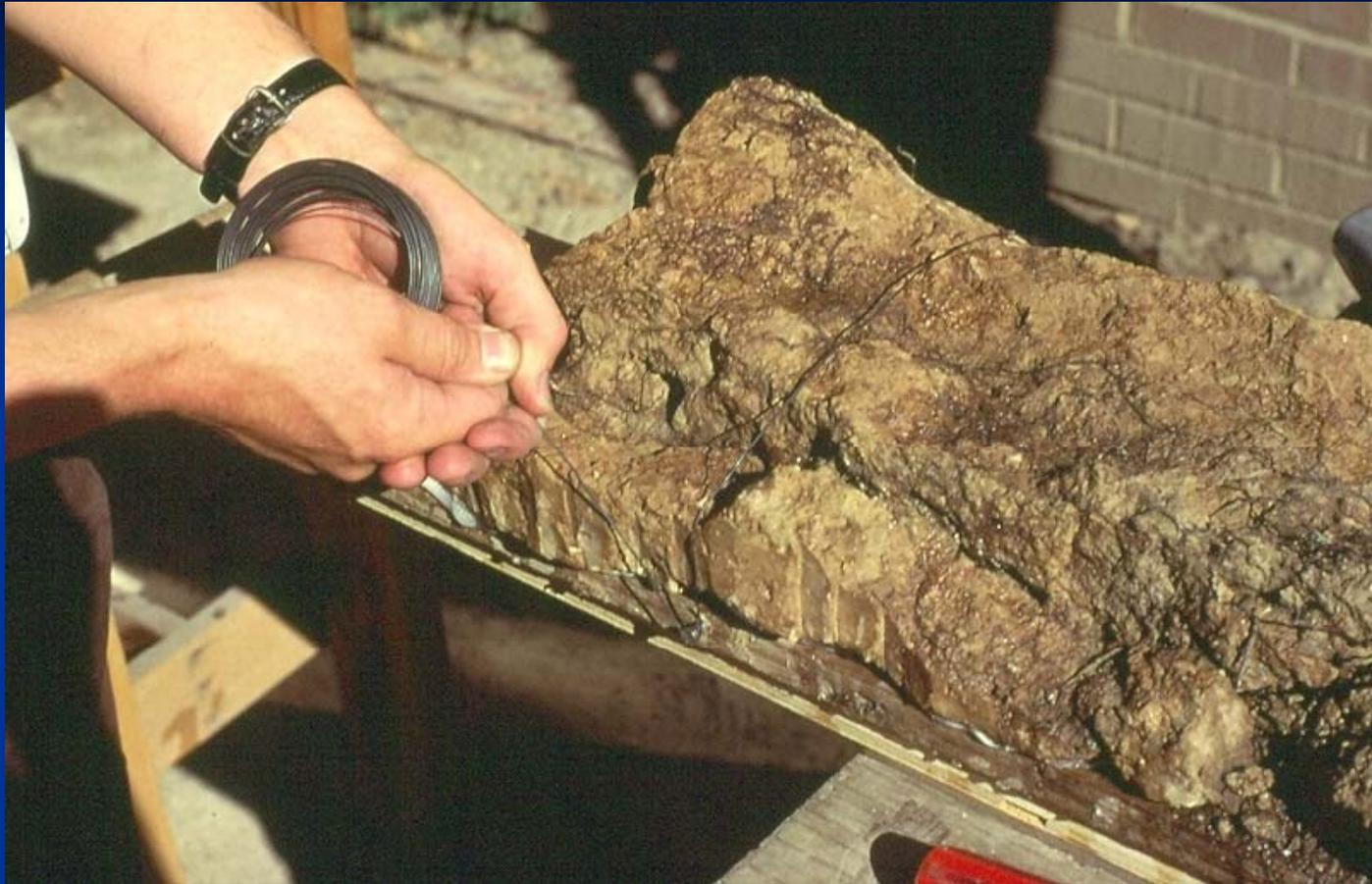
Use black soft iron wire to provide additional support for thick soils.
