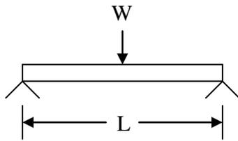
Simple Beam with Point Load
