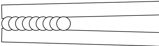
2. A 2" weld is made. As the weld progresses heat is transferred to the metal causing expansion forces which results in the pieces spreading apart.
