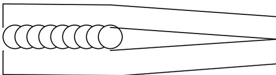
3. When the weld is stopped the deposited weld metal cools and contraction forces pull the two pieces of metal together, closing the gap.
