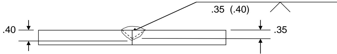
The effective throat measurement will be given in parentheses, left of the weld symbol.
