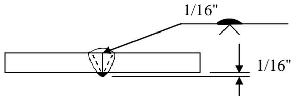
7. Surfacing and Hardfacing Welds – Welds that are applied to areas that need to be built up or need hardfacing to prevent wear. The height of the weld will be indicated to the left of the weld symbol.
