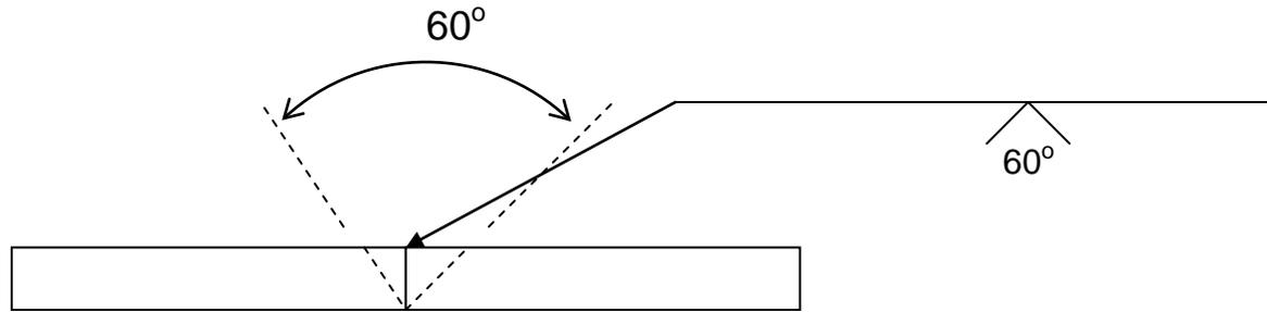
No measurement on depth, the Bevel goes all the way to the other side.
