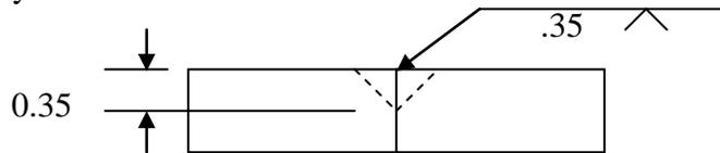
3. If a number appear in parentheses (.40) before the weld symbol, it will determine the depth of the effective throat.
