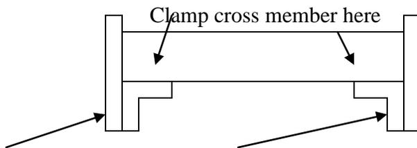
Clamp angle iron to frame here on both ends and in the center.
