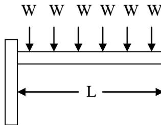
Cantilever Beam with Distributed Load
