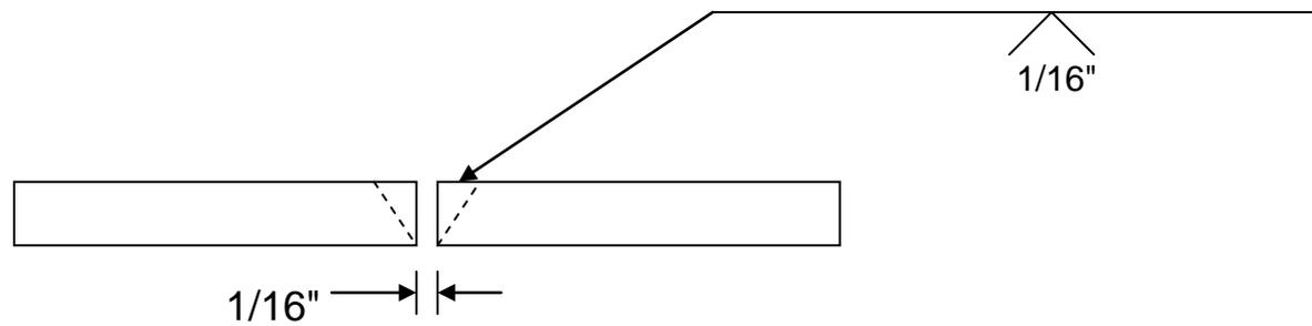
Gaps between the metal will be indicated on the weld symbol.
