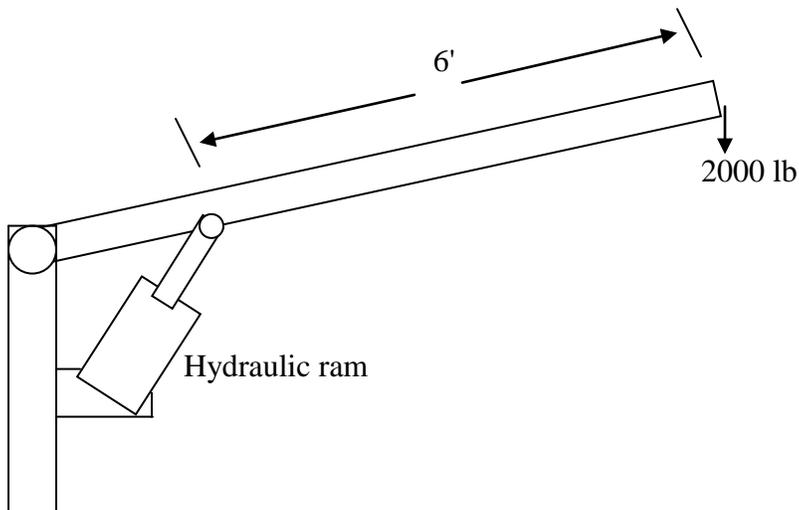
1. This is a cantilever beam with a point load. The shortest end of the beam is ignored because: It is shorter than the other end and it is a simple beam so it will have a lower moment than the other end. Therefore, if the long end is built to withstand the load the short end will have no problem withstanding the load.
