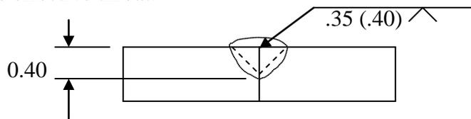
4. If a gap between the two pieces of metal is needed, it will be indicated on the weld symbol.
