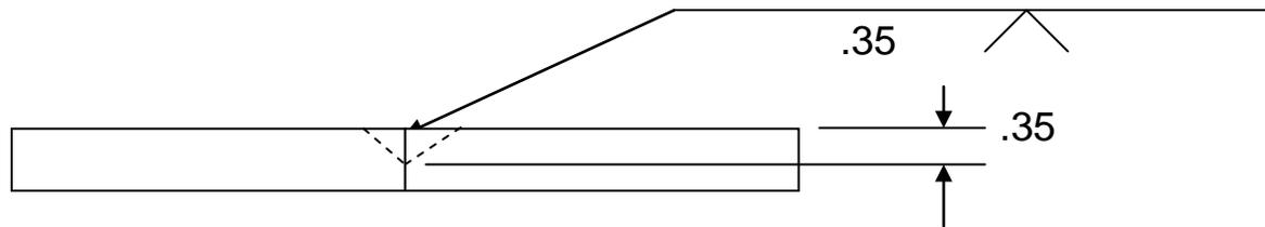
Measurements left of the weld symbol will indicate the depth of the groove.
