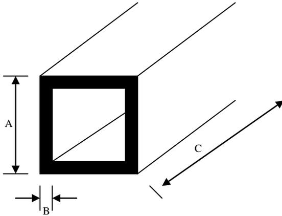
9. Rectangular Tubing-Longest outside dimension (A) given first, followed by shortest outside dimension (B), then wall thickness (C), finally length (D)
