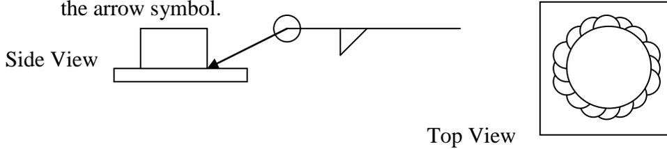
2. Field Weld, Symbol – When a weld is to be made or inspected out in the field a flag will appear on the reference line's connection with the arrow symbol.
