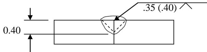
4. If a gap between the two pieces of metal is needed, it will be indicated on the weld symbol.
