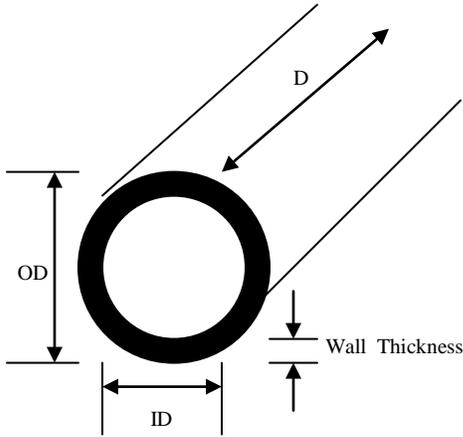
7. Round Mechanical Tubing-Outside diameter (OD) given first, followed by wall thickness (decimal inches, fractional inches, or wire gauge #), then length (D). See above illustration.
