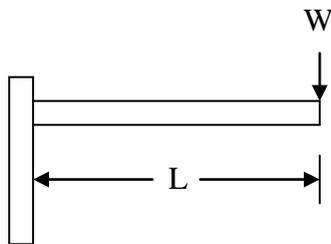
Cantilever Beam with Point Load
