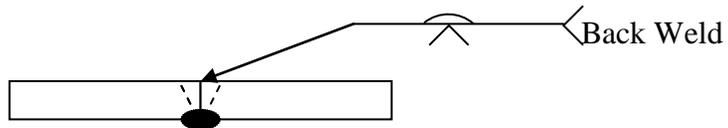
6. Melt-Through Welds – Welds that are required to melt through to the other side of the metal will be indicated by the melt-through symbol, which will appear opposite of the weld symbol. The height of the melt through will be indicated left of the melt-through symbol.
