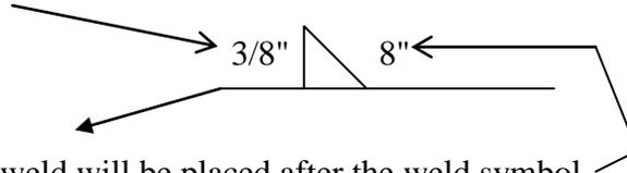
4. The length of the weld will be placed after the weld symbol.
