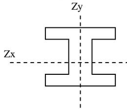
The bending moment must be calculated to determine safe load. There are two basic types of beams used to calculate bending moment. These are a simple beam (a beam supported on both ends) and a cantilever beam (a beam only supported on one end).
