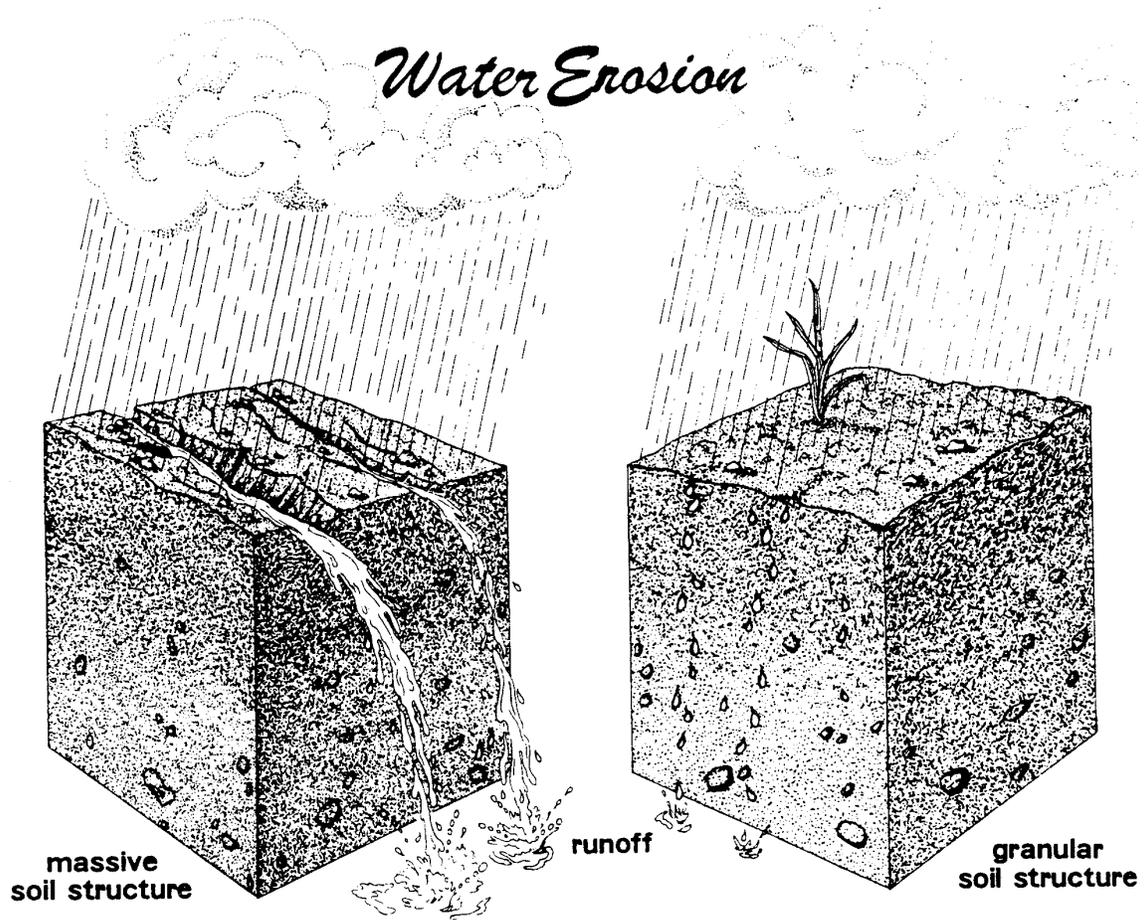
**infiltration rate affects erosion due to runoff**
