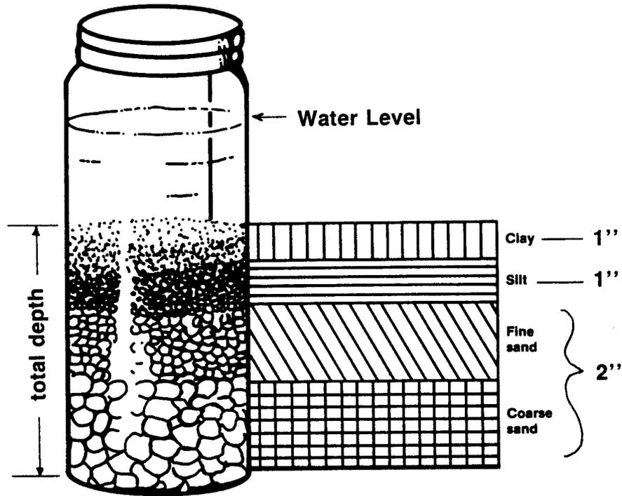
K. Determine the soil textural classification by using the soil textural triangle (Figure 2)
