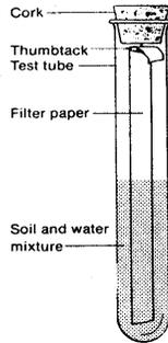
**b. Setup for isolating decomposers**
