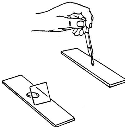
3. Holding a coverslip at a 45° angle, slowly lower it into the drop of water containing the letter. Preparing a slide in this manner is known as a *wet mount*. If properly done, there should be no air bubbles trapped under the coverslip. If this is not the case, start over again.
