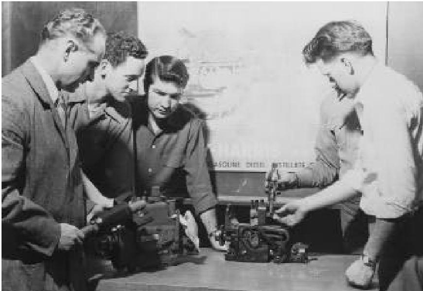
Agricultural Engineering students with model of a fuel injection system for a diesel tractor.
