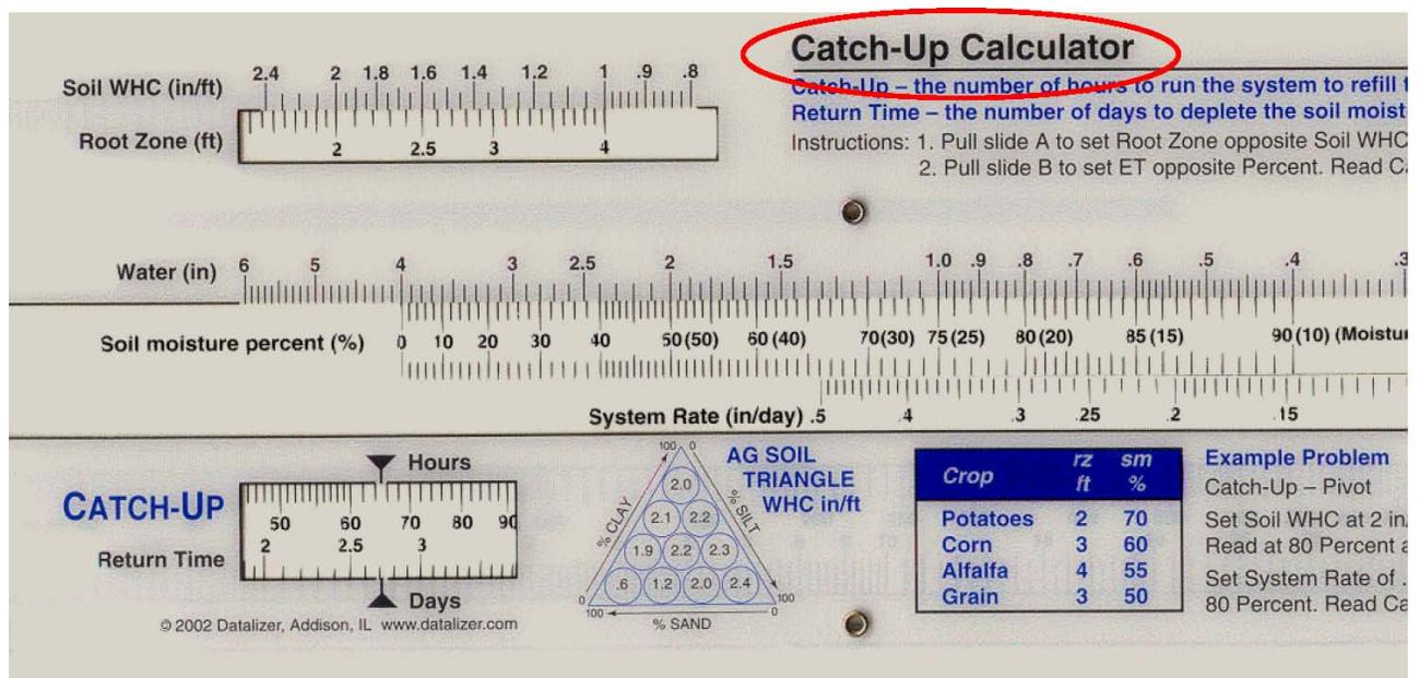
Figure 6. Catch up calculation for center pivot and linear move systems.
