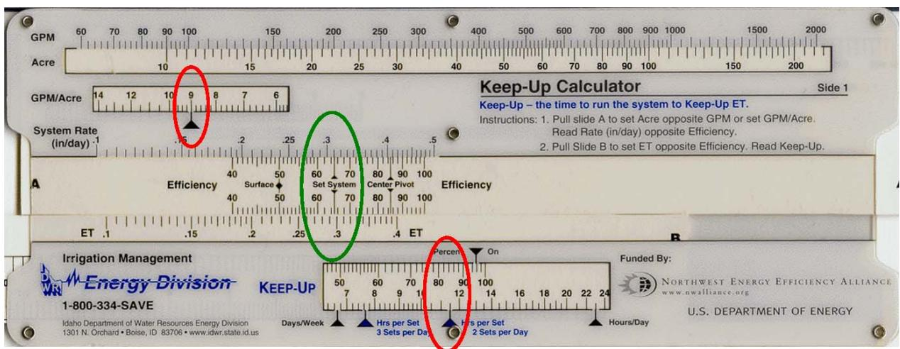
Figure 4. Irrigation interval for 11.5 hour sets on hand line and wheel line.
