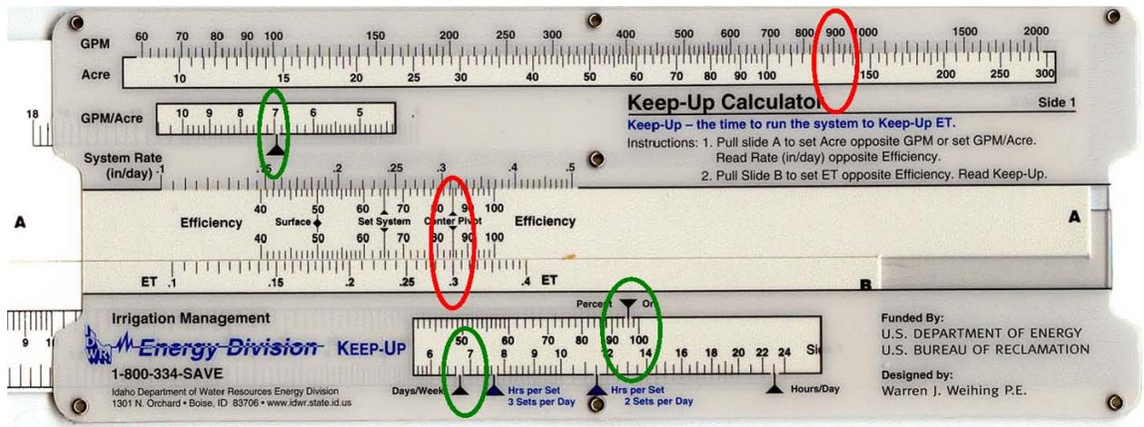
Figure 5. Keep-Up calculation for center pivot and linear move systems.
