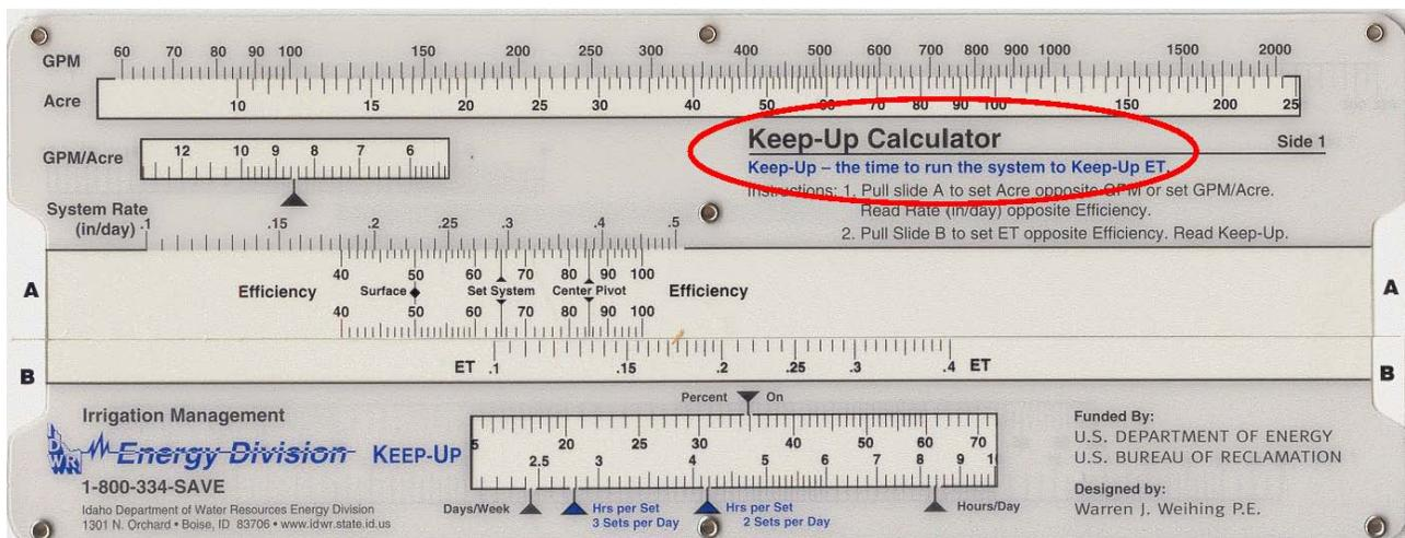
Figure 2. Keep-up side of slide rule.
