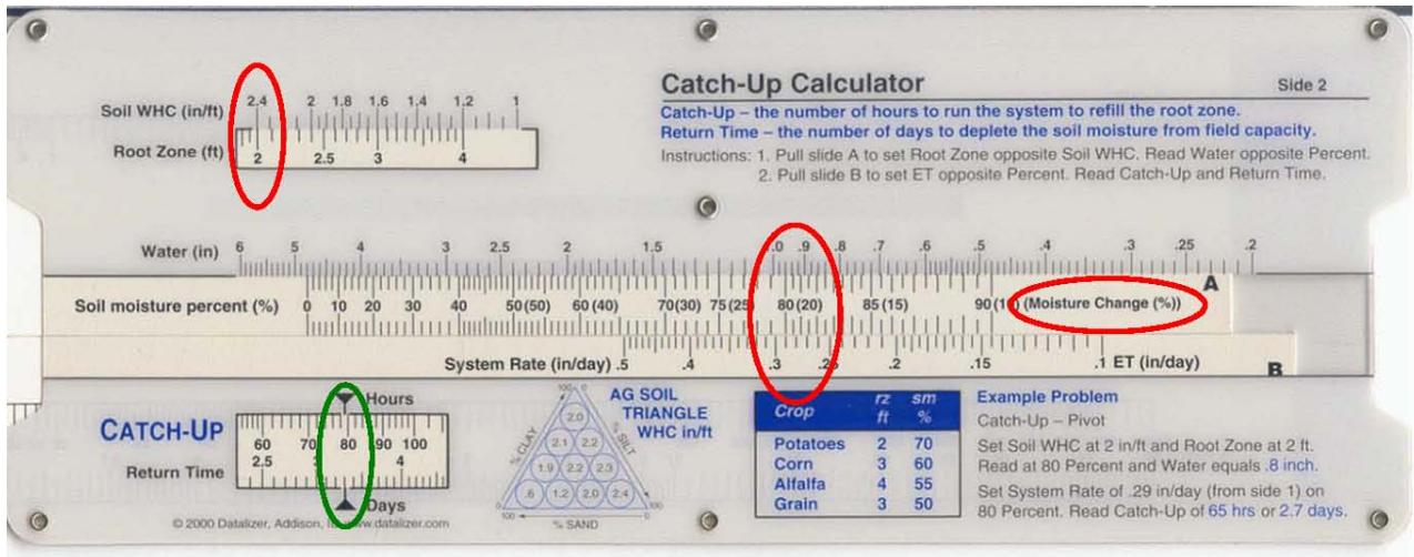
Figure 8. Catch-up slide rule silt loam example.
