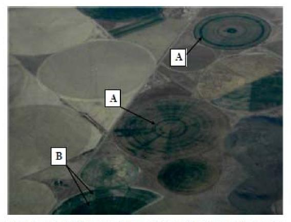
Figure 5. Poor center pivot uniformity due to malfunctioning pressure regulators (A) or incorrect nozzles on spans (B)
