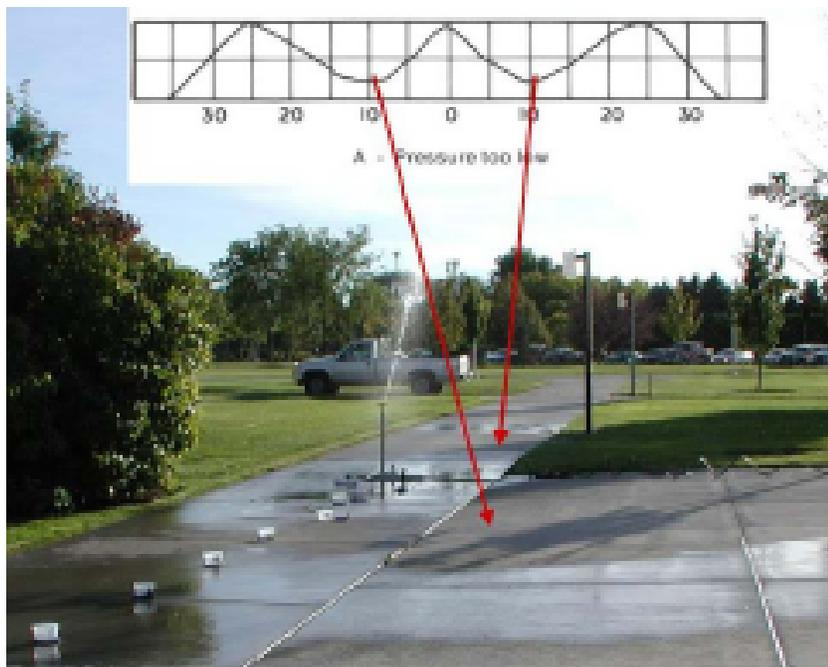
Figure 12. Water distribution from a sprinkler test using a brass nozzle at 20 psi system pressure for 20 minutes. Note the dry areas on the pavement corresponding to low areas in the theoretical distribution shown above.
