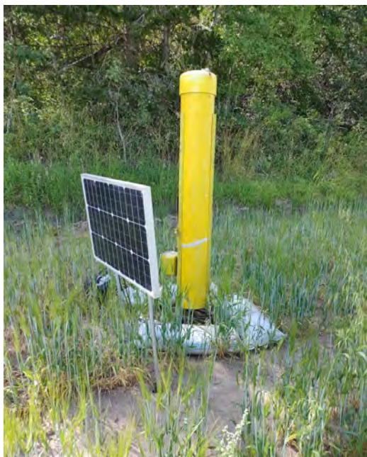
Figure 2. A suction trap, approximately six feet tall, located at the edge of a potato field. It is powered by a battery and solar panel. Suction from a fan forces insects into a 50% PEG-filled glass jar, where they are trapped.
