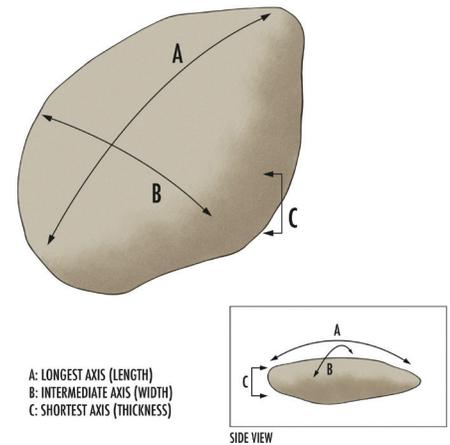
Figure 33. In a Wolman pebble count, you will measure the B-Axis of the pebbles, which is the midlength axis. *Courtesy of Noah Kroese..*
