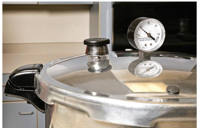
**Figure 19.** Allow the canner to depressurize normally without assistance.
