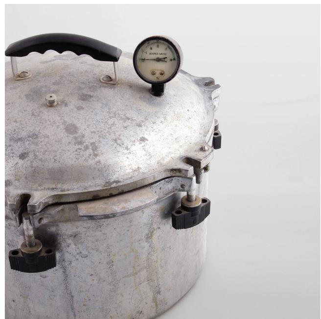
**Figure 10.** Pressure canner with corrosion and pitting.
