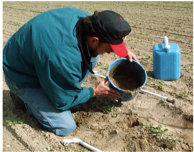
Figure 7. Pouring soil slurry into sensor holes.
