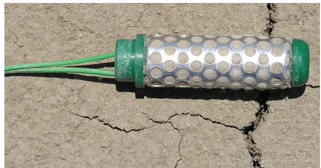
Figure 1. Watermark soil moisture sensor.
