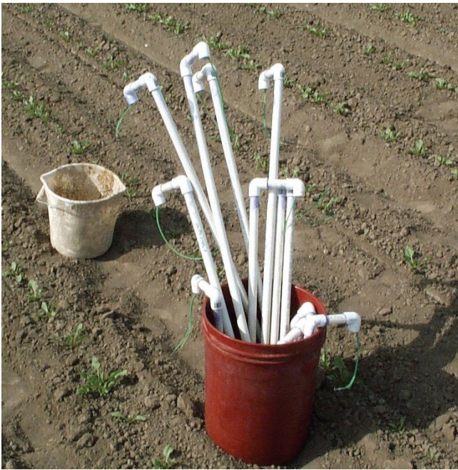
Figure 6. PVC-mounted sensors ready for installation.
