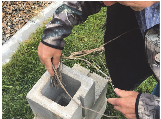
Students learned how to make rocket stoves with cinder blocks for outdoor cooking and warmth. Photo credit: Lance Ellis.
