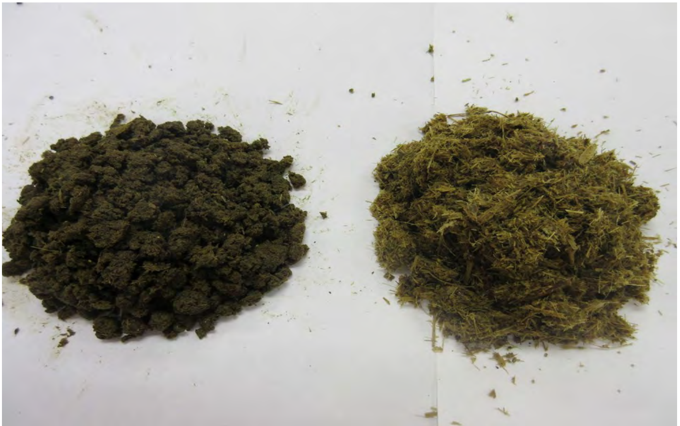
Figure 1. Centrifuge separated solids (left) vs. screen separated solids (right).
