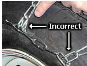
2. Double-check to make sure that the sharp, open-hook side of the tire chains is facing down. Otherwise, if the hooks are facing up, they will eventually face toward the tire after the chains are installed, which may cause tire damage.
