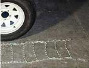
1. Lay chains out flat and remove all twists and tangles. Arrange chains so that the side with the sharp open hooks is facing down and away from the tire.
