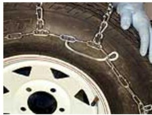
9. Pull bow lever past link, insert into link, and release. After lever is hooked, check chains for a good, tight fit. Make sure chains are centered on tire, with the same number of free links on the inside and outside.
