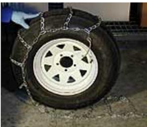
5. Drive tire over the top of chains so that the bow-lever side of the chains is on the outer side of the tire and the "C"-hook side of the chains is on the inner side of the tire. Leave about 1 foot of chain off the tire as shown in the picture at the left.
