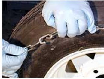
6. On the inner side of the tire, take the "C" hook and hook it through the chain link on the other end of the chains.
