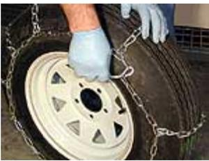
8. Then pull back on the bow lever. This will tighten the chains.
