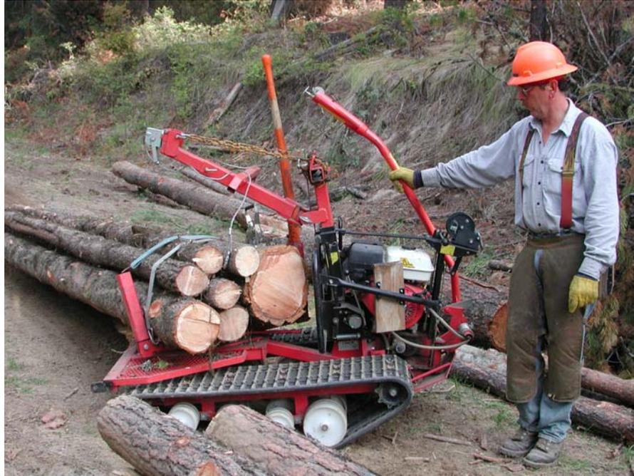
**Figure 6. Typical Iron Horse log load**
