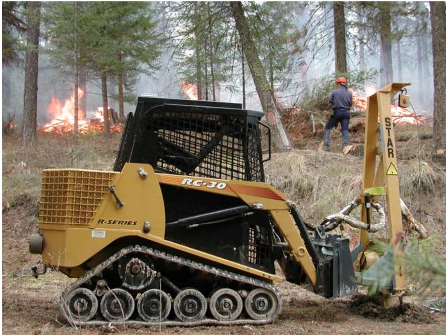
**Figure 7. ASV RC30 with radio remote control log winch**
