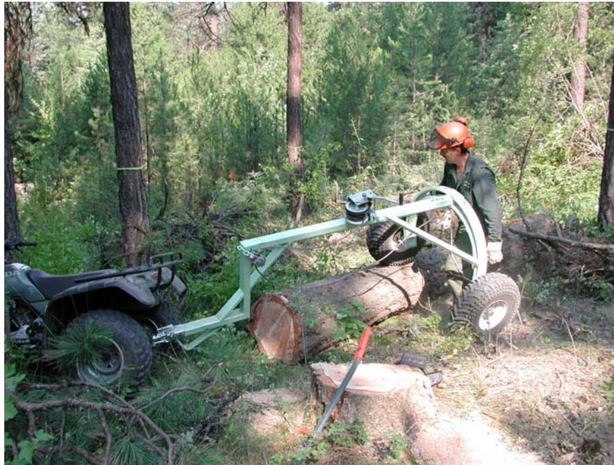
**Figure 5. Positioning the ATV arch over log**
