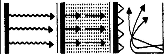
fireplace walls into the house, and warm house air is pulled into the fireplace by convection and goes up the chimney. The ideal fireplace will maximize the radiation and the convected heat it emits, and minimize the amount air escaping up the chimney (Figure 2).
