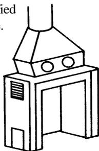
A manufactured unit known as the zero clearance fireplace is insulated so that it can be placed directly against combustible walls and floors. The insulation usually consists of an air chamber that opens to the outside by the chimney.
