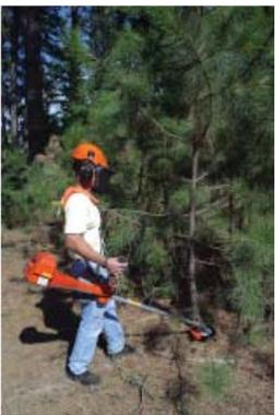
Depending on the job, a variety of tools can be used for mechanically controlling brush, ranging from loppers and pruning shears on smaller jobs, to chainsaws or clearing saws for multiple stems or stems larger than 1 inch. For smaller diameter stems, brush mowers, brush hogs, or similar devices may be used. Regardless of the
