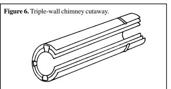
**Prefabricated Metal Chimneys.** Prefabricated chimneys are easier to erect than masonry ones. Tests of the National Bureau of Standards have shown that metal and masonry chimneys differ little with respect to draft when used under similar conditions. Metal prefabricated chimneys must be UL listed "All Fuel" since others are not insulated or vented enough for wood burning. Wood stove flue gases get hot enough to melt the aluminum alloy use din chimneys designed for gas appliances.
