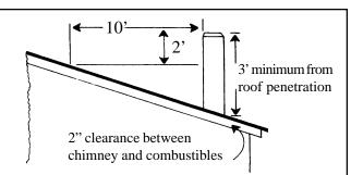
**Figure 2.** To prevent downdrafts and fire from sparks, chimney height must be at least 2 feet above any roof surface within 10 feet horizontally.
