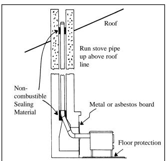
**Figure 3.** When attaching a small stove to a fireplace, run the stove pipe up into the chimney above the damper. extend the stove pipe above the roof line if there is no flue liner or if the flue is very large. Use fiberglass or rock wool for sealing.
