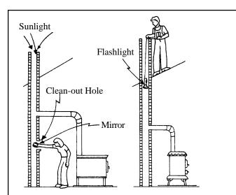
**Figure 1.** The chimney may be inspected from the roof or, in some cases, a mirror can be used to look up through the chimney flue, provided the chimney is straight. If you use an air-tight stove, check the stove pipes once a month.
