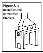
A manufactured unit known as the zero clearance fireplace is insulated so that it can be placed directly against combustible walls and floors. The insulation usually consists of an air chamber that opens to the outside by the chimney. The cool air circulating around the unit is the insulation. Mobile homes often use zero clearance unit since they require less bulk and weight to install.
