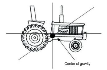
**Base of stability** is defined as the area within the points where the tractor's wheels contact the ground. The base of stability depends upon the front- and rearwheel spacing and the axle-to-axle spacing.
