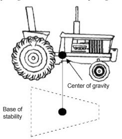
As long as the tractor is operated so that its center of gravity is within the base of stability, the tractor will not roll over.
