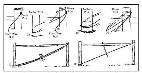
Figure 12. Correct procedure for threading the nine gauge smooth wire used as diagonal in the brace assembly.
