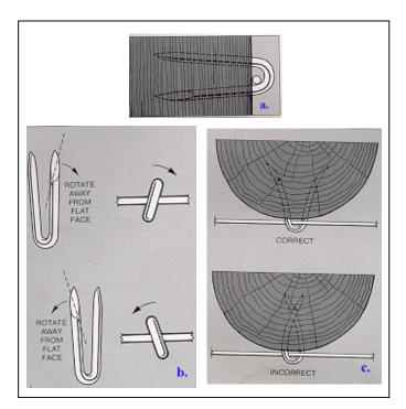
Figure 16. Proper stapling techniques.
