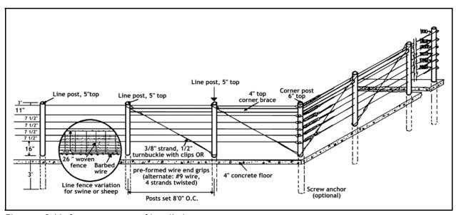
Figure 7. Cable fence — one type of installation.
