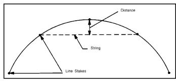
Figure 10. Fence post spacing around curves.
