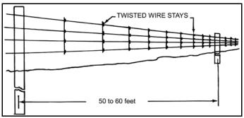
Figure 5. Typical barbed wire suspension fence.
