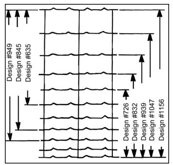
Figure 6. Some common woven wire designs. Standard design numbers describe the wire: 949-12-11, for instance, means the fence has 9 horizontal wires and is 49 inches high; has 12-inch spacing of stay (vertical) wires and 11-gauge stay and intermediate wires. (Top and bottom wires are usually two sizes larger.)
