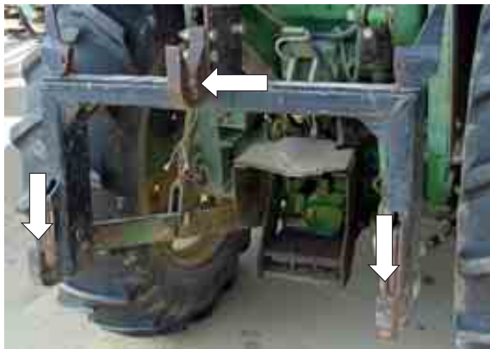
Figure 5. ASAE standard category 1 quick hitch mounted on a compact tractor. Notice three points of attachment to implement.
