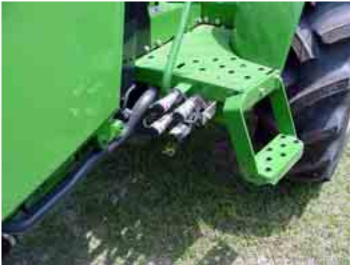
Figure 11. Remote hydraulic outlets near operator's foot
