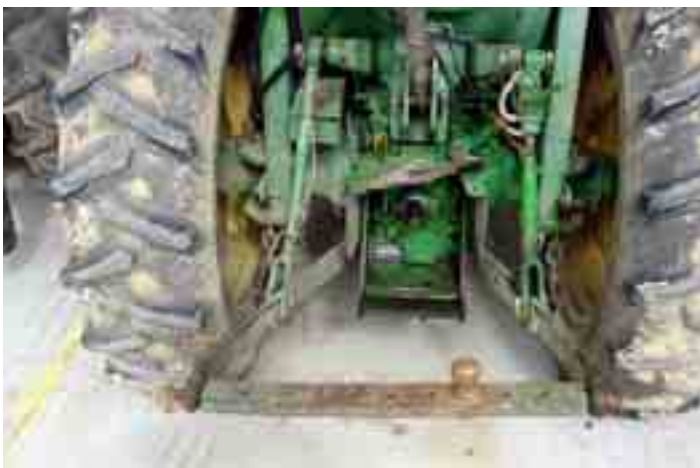
Figure 9. Drawbar mounted to 3-point hitch. Note: this setup is unsafe and NOT recommended.
