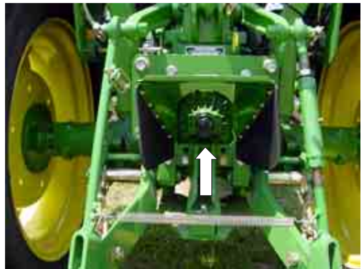
Figure 10. 540-rpm PTO shaft on compact tractor
