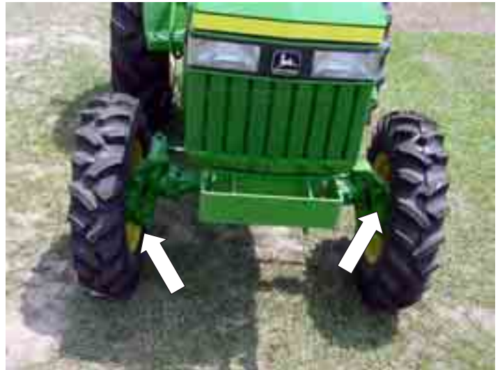
Figure 16. Front wheel assist (FWA) on compact tractor
