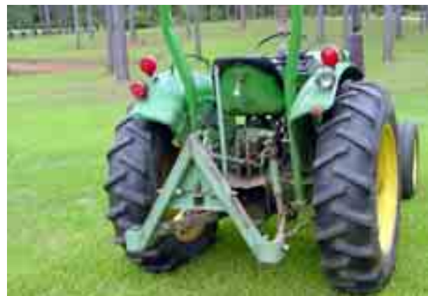
Figure 6. Delta-shaped category 1 quick hitch mounted on a compact tractor.
