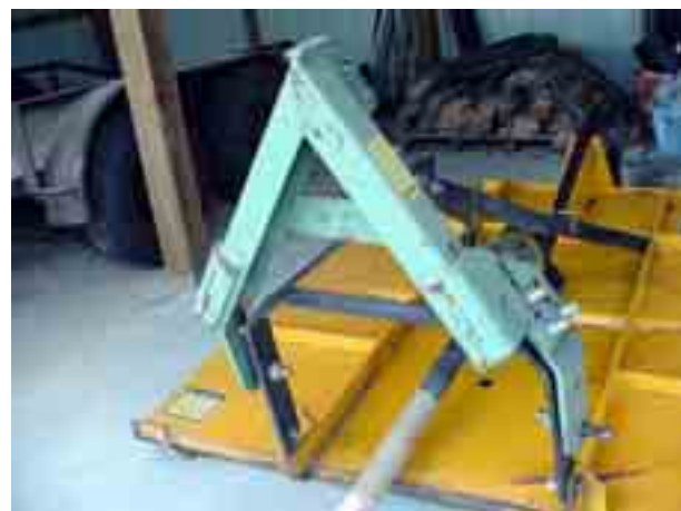
Figure 7. Implement portion of delta-shaped category 1 quick hitch
