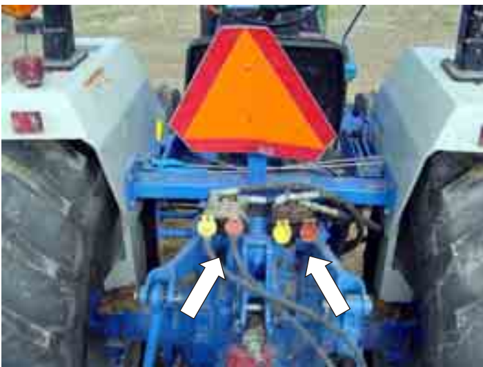
Figure 12. Remote hydraulic outlets extended to rear of compact tractor
