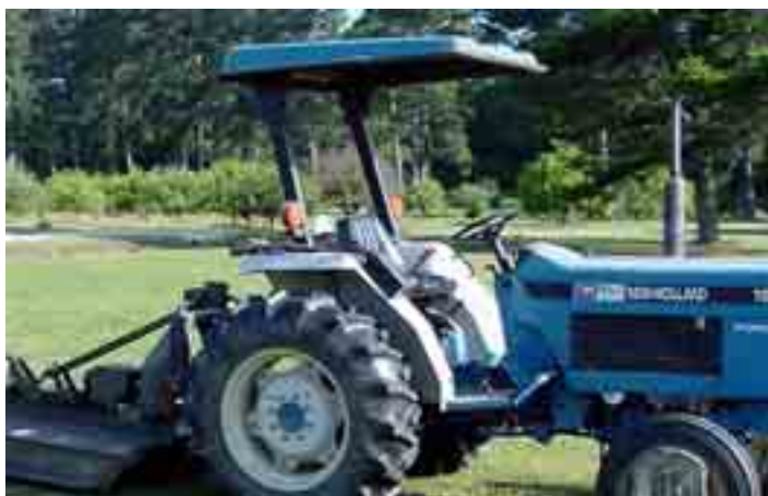
Figure 3. Rollover protective structure (ROPS) on compact tractor
