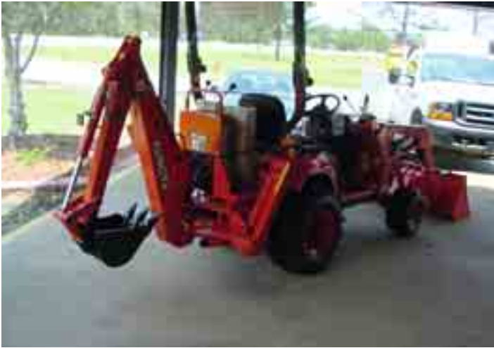
Figure 24. Backhoe and front end loader on compact tractor
