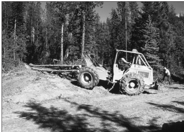
Figure 15 — The typical rubber-tired skidder will provide very economical yarding in a variety of silvicultural prescriptions. The use of a cable winch and chokers as shown in this picture increases machine versatility and reduces soil compaction compared with using the same machine equipped with a grapple.
