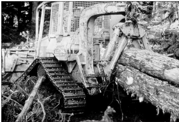
Figure 13 — A crawler tractor is among the most versatile of machines. When equipped with winch and chokers or a grapple as shown in this picture, it can be used for yarding. Wide, low ground pressure tracks reduce soil compaction.
