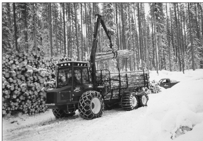
Figures 9 & 10 — A method of commercial thinning now becoming common is the use of a harvester-forwarder combination in what is called a cut-to-length system. The harvester moves through the stand felling, delimiting, bucking and bunching trees selected for harvest (Figure 9); meanwhile a forwarder loads and moves these processed logs to the truck road where it then unloads and sorts the logs into decks for log truck pickup (Figure 10).
