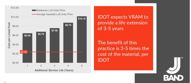
41 Improving HMA Pavements with a Void Reducing Asphalt Membrane
