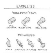
**Pre-molded earplugs** do not need to be rolled to conform to a worker's ear canal but the right sized earplugs must be used. They are relatively inexpensive, reusable, can be washed, require less handling, and come in a variety of sizes.
