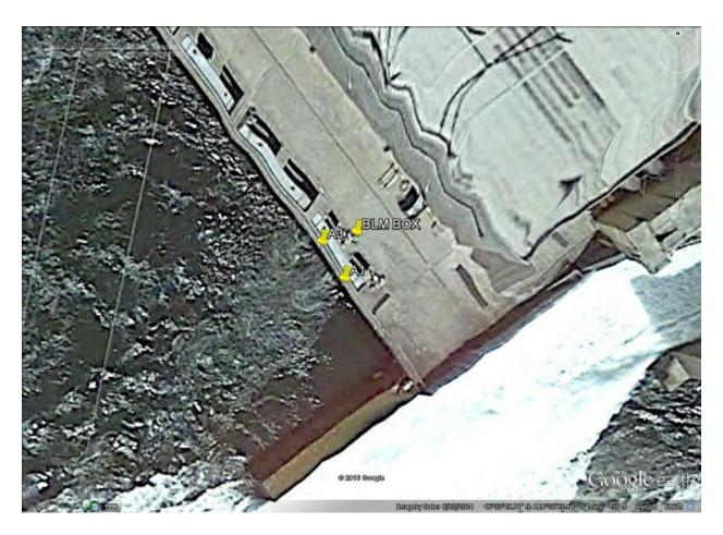
BLM A1 and A3 and receiver box locations. A2 and A4 are inside under deck.
