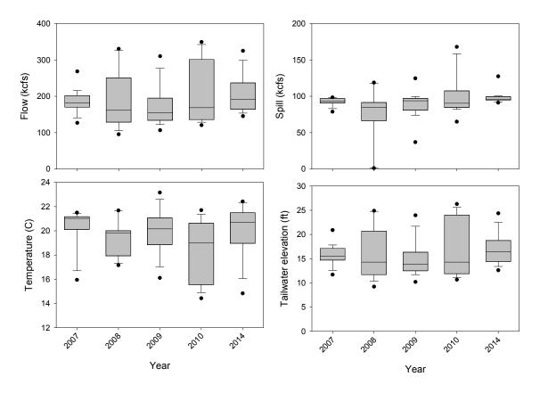
Figure 28. Box plots of the total discharge ('flow'), spill, temperature, and tailwater elevation on the days that radio-tagged adult lamprey first approached the CI. Distributions show 5<sup>th</sup>, 10<sup>th</sup>, 25<sup>th</sup>, 50<sup>th</sup>, 75<sup>th</sup>, 90<sup>th</sup>, and 95<sup>th</sup> percentiles.
