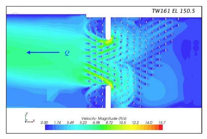
Figure 36. Velocity contours on horizontal plane (6" above invert) with elongated, rotated bollard configuration at the John Day north entrance. Q = flow direction (Source: Yin et al. 2010).
