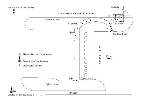
Figure 4. Diagram showing radio antenna deployments at Bonneville Dam PH1 and B-Branch fishways in 2014 (not to scale).
