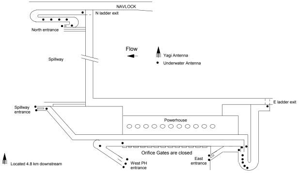
Figure 6. Diagram showing radio antenna deployments at The Dalles Dam in 2014 (not to scale).
