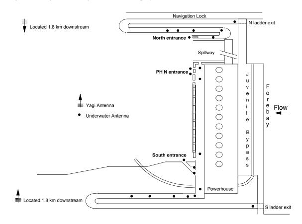
Figure 7. Diagram showing radio antenna deployments at John Day Dam in 2014 (not to scale).
