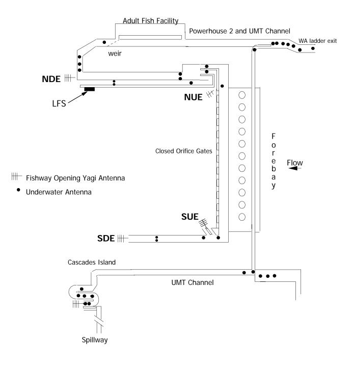
Figure 5. Diagram showing radio antenna deployments at Bonneville Dam PH 2 and Cascades Island in 2014 (not to scale). See Figure 9 for LFS details.
