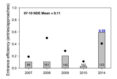
Figure 18. NDE (gray bars) and SDE (solid circles) entrance efficiency estimates (total entry events/total approach events) for radio-tagged lamprey during nighttime (22:00-04:00 h) with reduced velocity conditions (except in 2008). Samples sizes in each bar are the numbers of lamprey that approached NDE.
