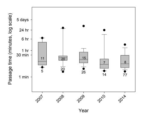
Figure 23. Lamprey passage time distributions (plotted on log-scale) from NDE to the antenna at the base of the ladder. Numbers inside boxes are median times in minutes. Distributions show 5<sup>th</sup>, 10<sup>th</sup>, 25<sup>th</sup>, 50<sup>th</sup>, 75<sup>th</sup>, 90<sup>th</sup>, and 95<sup>th</sup> percentiles; sample sizes are below boxes.
