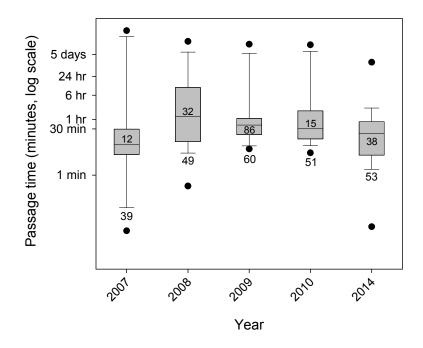
Figure 27. Lamprey passage time distributions (plotted on log scale) from approach to entry at Cascades Island fishway. Values inside boxes are median times in minutes. Distributions show  $5^{\text{th}}$ ,  $10^{\text{th}}$ ,  $25^{\text{th}}$ ,  $50^{\text{th}}$ ,  $75^{\text{th}}$ ,  $90^{\text{th}}$  and  $95^{\text{th}}$  percentiles; sample sizes are shown at bottom.
