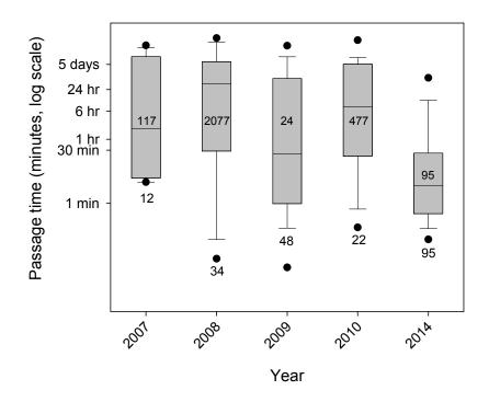
Figure 20. Radio-tagged lamprey passage time distributions (log scale) from approach to entry at the Bonneville NDE. Values inside boxes are median times in minutes. Distributions show 5<sup>th</sup>, 10<sup>th</sup>, 25<sup>th</sup>, 50<sup>th</sup>, 75<sup>th</sup>, 90<sup>th</sup> and 95<sup>th</sup> percentiles; sample sizes are shown at bottom.
