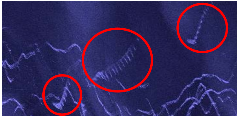
Figure 4. Example of tail-beat frequency (TBF) patterns generated from the echogram procedure in the DIDSON v5.25.25 software. The y-axis depicts range (distance from camera) and the x-axis represents time (frame number). Brightness indicates intensity of reflected acoustic signals. The echo traces of three lamprey from the JPU_LONG deployment are shown in this figure (enclosed by red circles). The “spikes” in each example represent the position of the lamprey’s body as it undulates from side to side. The time difference between the peaks of each successive spike provides information about the rate at which the body is undulating. The greater the time between peaks, the shorter the TBF estimate.
