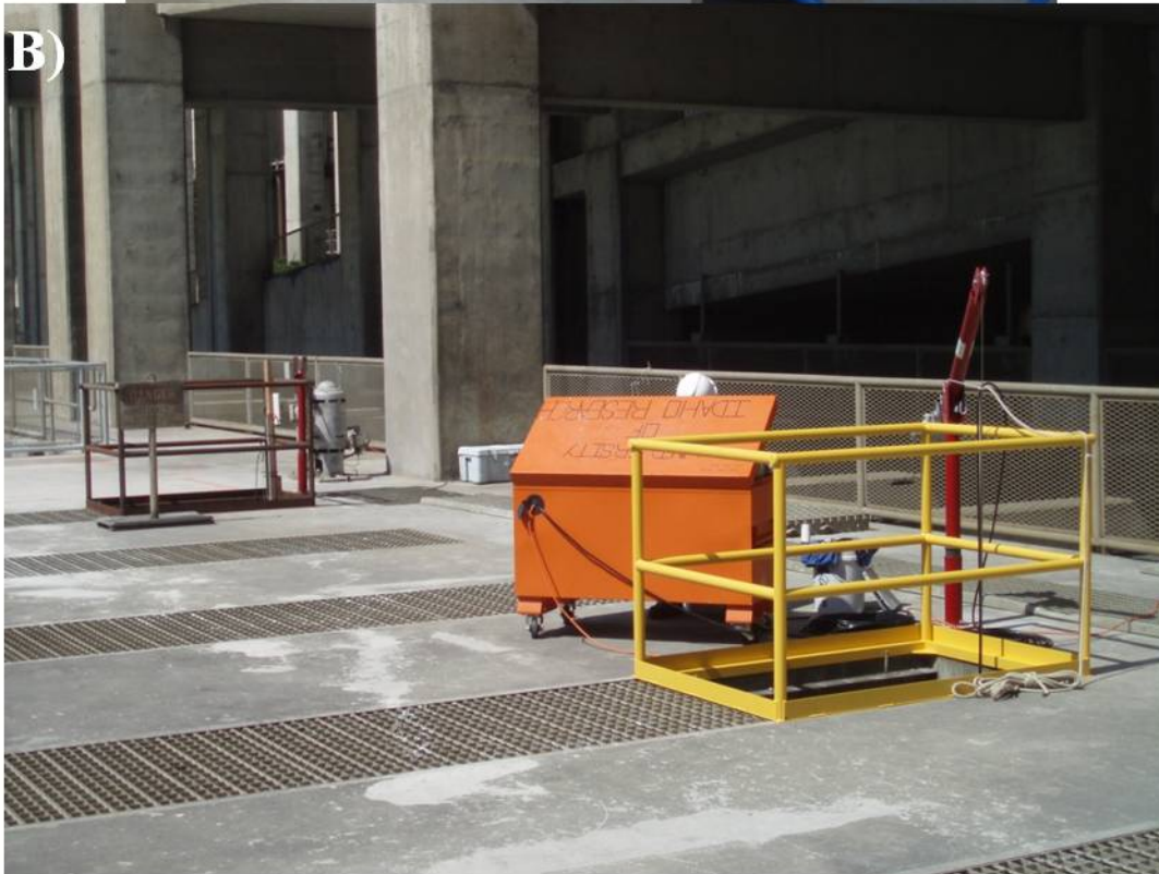
Figure 8. (A) DIDSON camera attached to the aluminum trolley at JD4 and (B) typical set up with the davit and protective workbox at John Day Dam.
