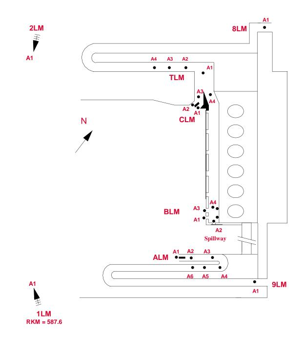
Figure 5. Locations that radiotelemetry antennas were deployed inside the Lower Monumental Dam fishway in 2013. (Not to scale.)
