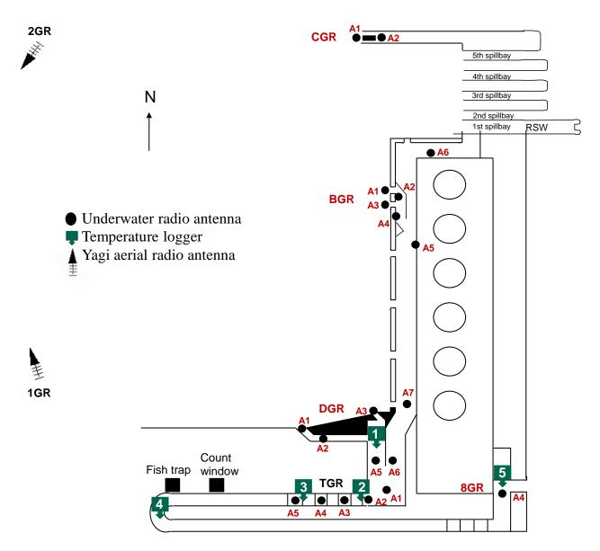
Figure 7. Locations that water temperature loggers and radiotelemetry antennas were deployed at Lower Granite Dam in 2013. (Not to scale.) Temperature loggers: (1) south shore entrance, (2) lower transition pool, (3) upper transition pool, (4) above adult fish trap and (5) fish ladder exit.
