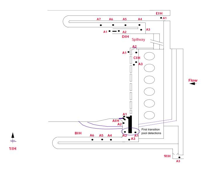
Figure 4. Locations that water temperature loggers and radiotelemetry antennas were deployed inside the Ice Harbor Dam fishway in 2013. (Not to scale.)
