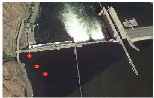
Figure 8. Location of temperature logger strings deployed in Lower Granite forebay in 2013.
