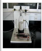
The reactor was moved from Moscow, Idaho, to the new laboratories in Boise, Idaho. The team calibrated a hot wire anemometer, used the anemometer to remeasure the plug-flow region of the reactor, and began testing and modeling of a platinum (Pt) wire catalyst exposed to a lean propane-oxygen-nitrogen mixtures.
