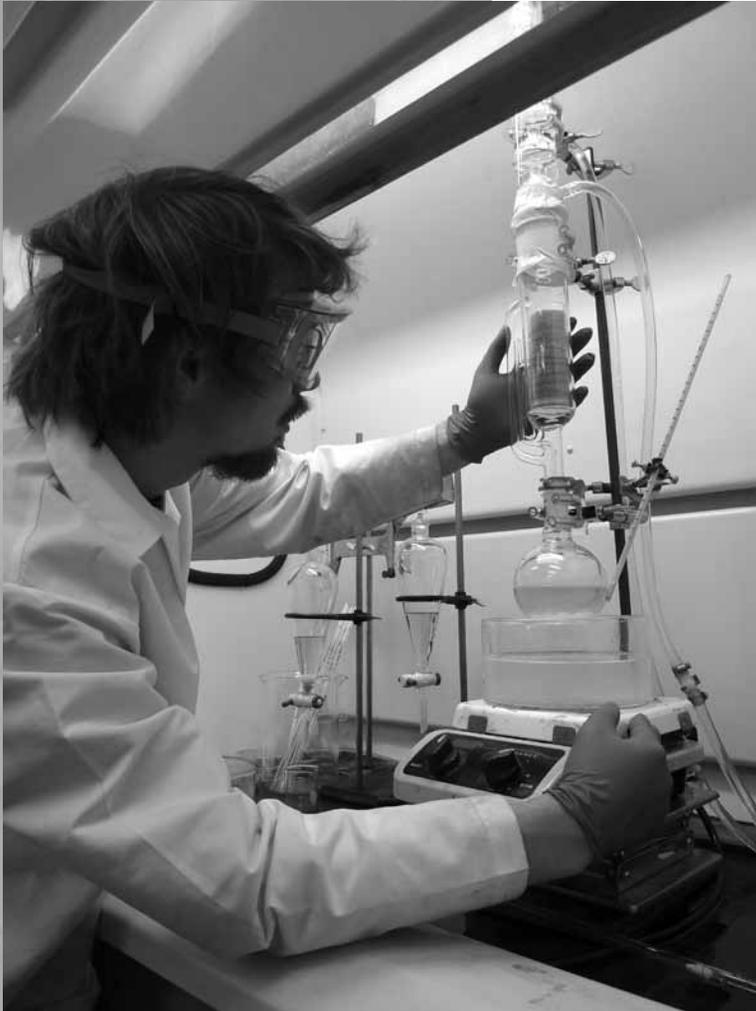
*Keegan Duff solvent extracts macerated Camelina Sativa seeds with dimethoxyethane ether using a soxhlet apparatus. Extracts are subsequently run through a preparatory column to isolate the glycolipids for qualitative and quantization.*
