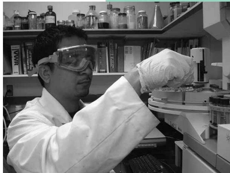
*Undergraduate student Sushant Kshetri prepares the samples collected from catalytic thermochemical conversion of glycerol to alcohols for gas chromatograph analysis.*
