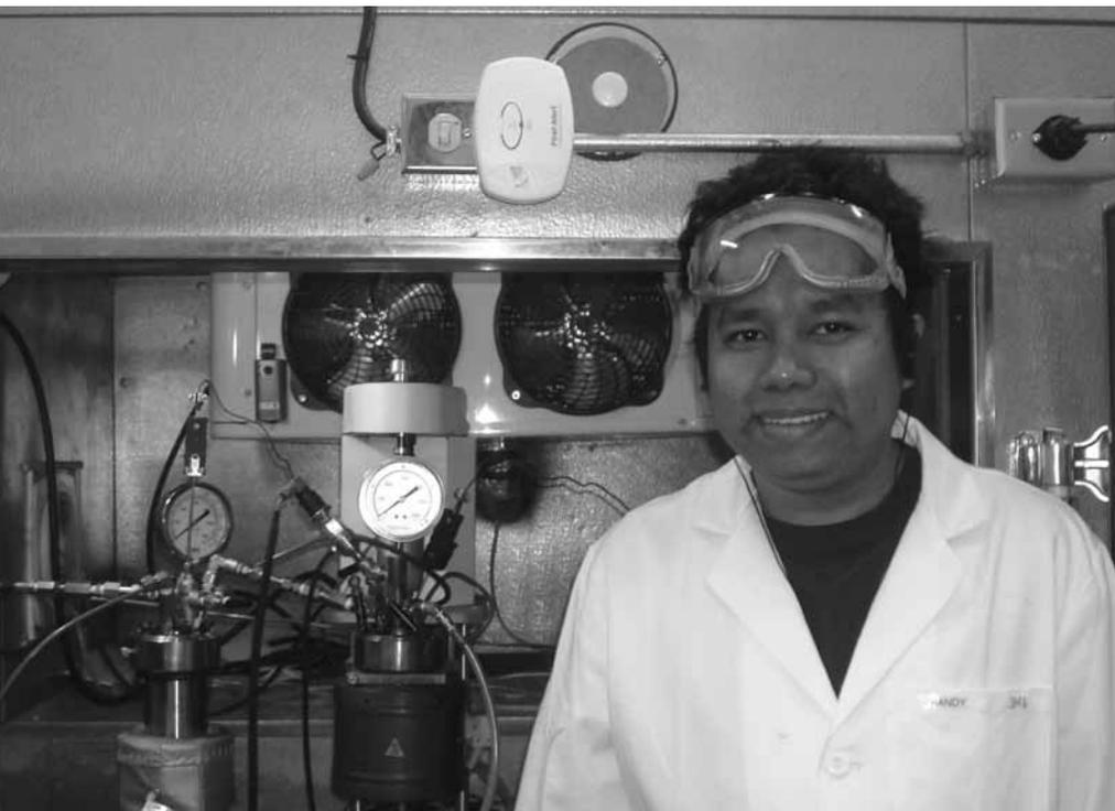
*Graduate student Randy Maglinao working on the reactor-feeder system for catalytic thermochemical conversion of glycerol to alcohols.*
