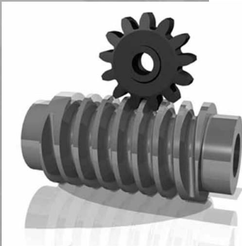
*Example of CATIA produced worm and spur gear combination.*
