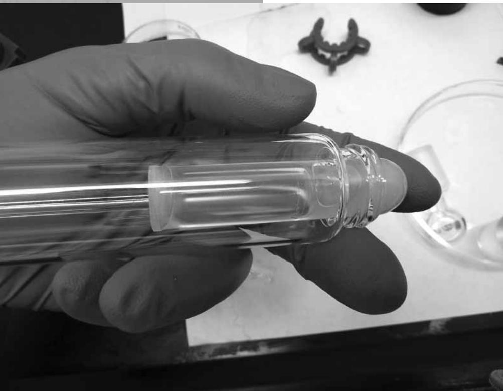
*A modified Craig tube is used for recrystallization of residues with significant sterol glucoside content dissolved in tetrahydrofuran.*
