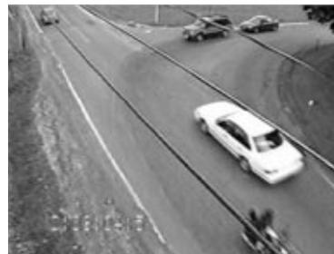
*Illustration from the Highway Capacity module showing a stop controlled T-intersection where the minor street left turn vehicles are waiting to accept a gap between the major street vehicles.*
