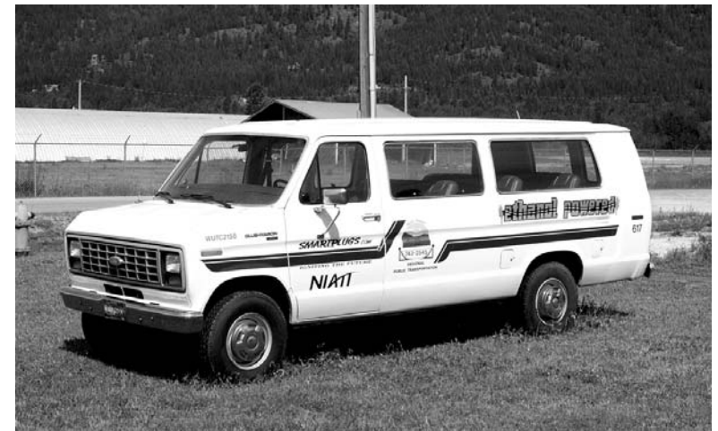
Valley Transit van converted to a dual fuel platform with catalytic igniters.
