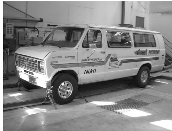
The chassis dynamometer in use.
