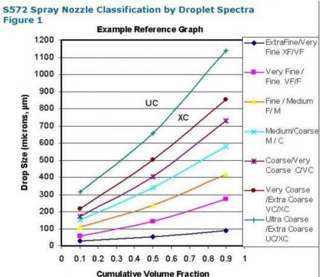
Sample reference graph developed from measurements averaged from three types of laser instruments
