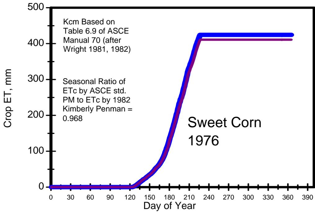
— using 1982 KPen      — using ASCE std.PM
