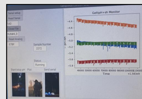
Figure 5: The program used for tracking the pH of the GellipHish's sinks and source.
