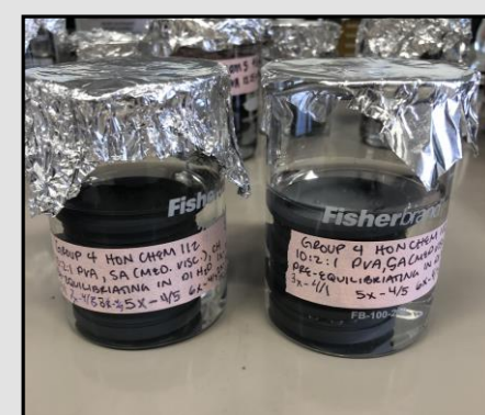
Figure 3: A set of hydrogel pucks equilibrating in DI water.
