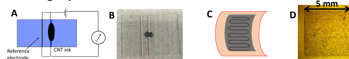
Figure 2. (A) Schematic of drop-casted glass slide (B) Drop-casted glass slide (C) Schematic of calcium ionophore-ink mix on flexible surface; (D) Calcium ionophore-ink mix printed on flexible Kapton® surface.
